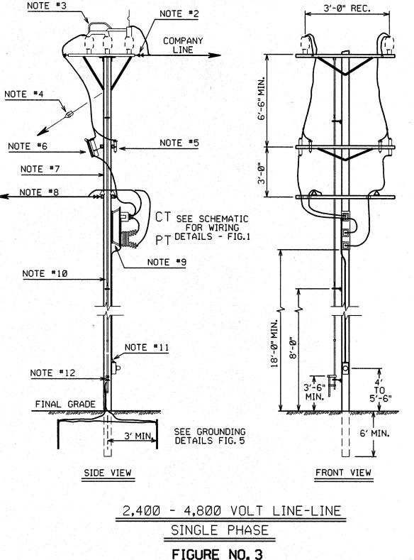
CUSTOMER'S OUTDOOR RECEIVING STRUCTURE ARRANGEMENT SINGLE-PHASE-100KVA LIMITATION
