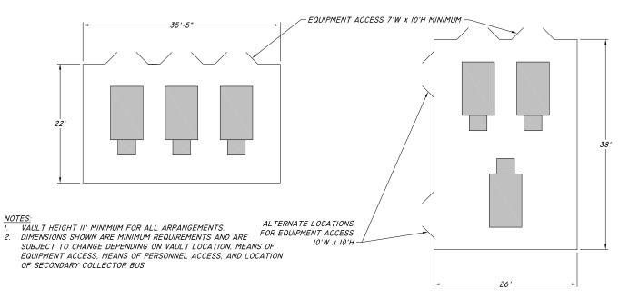
Figure 36 – Building & Free-Standing Vault Standard Arrangements, 3 – 2000 kVA, 23 kV
