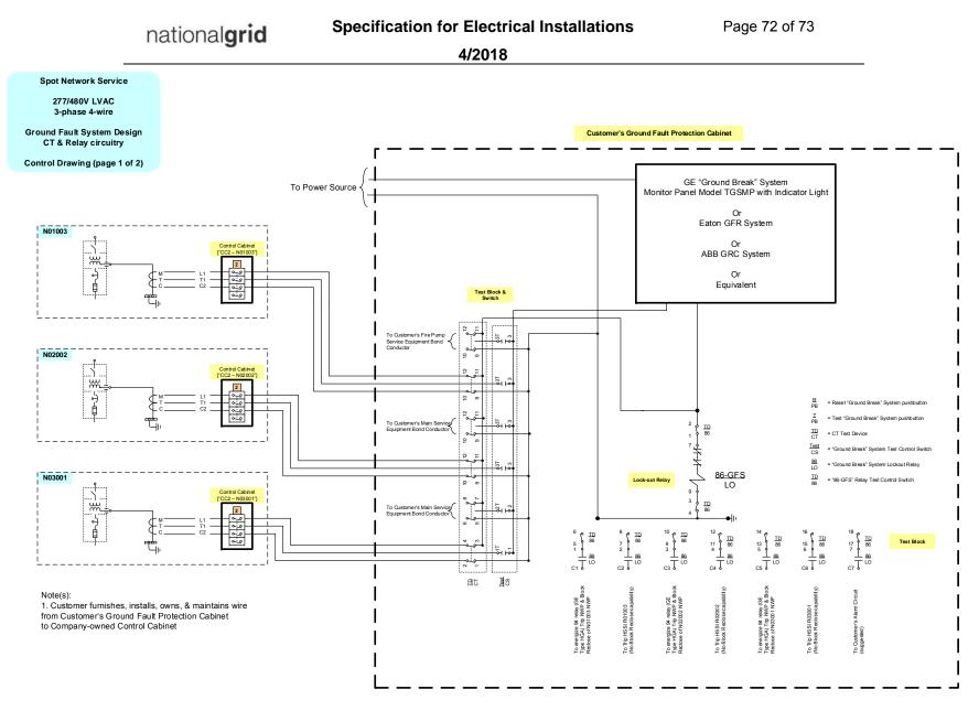
Figure 58 – Ground Fault Protection Control System Example Sheet 1
