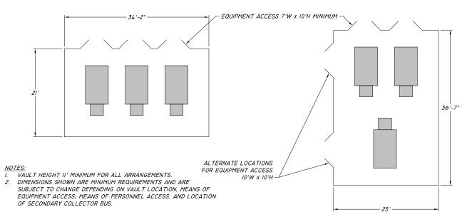
Figure 42 – Building & Free-Standing Vault Standard Arrangements, 3 – 1500 kVA, 34.5 kV
