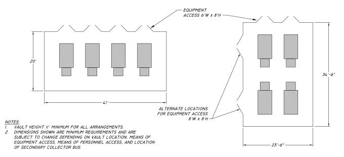
Figure 22 – Building & Free-Standing Vault Standard Arrangements, 4 – 1500 kVA, 15 kV
