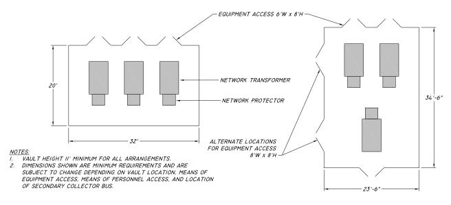
Figure 21 – Building & Free-Standing Vault Standard Arrangements, 3 – 1500 kVA, 15 kV
