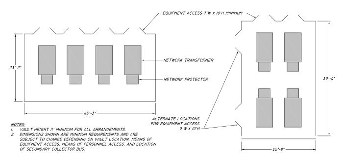
Figure 28 – Building & Free-Standing Vault Standard Arrangements, 4 – 2500 kVA, 15 kV
