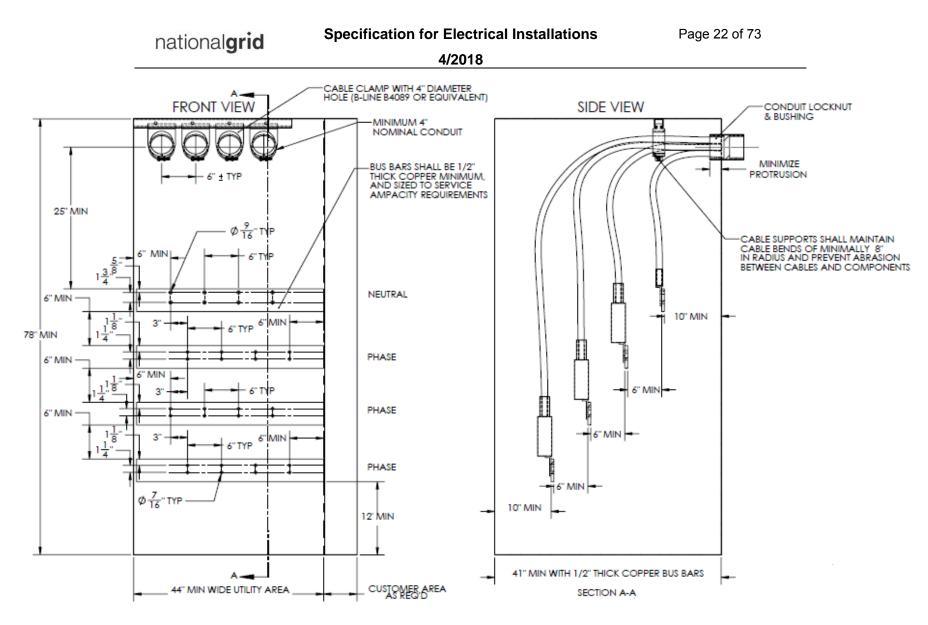
Figure 12 – 1000 to 1600 amperes Limiter Enclosure (Top Entry from Wall)
