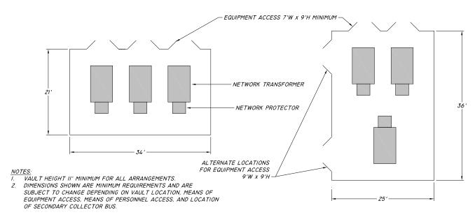
Figure 24 – Building & Free-Standing Vault Standard Arrangements, 3 – 2000 kVA, 15 kV
