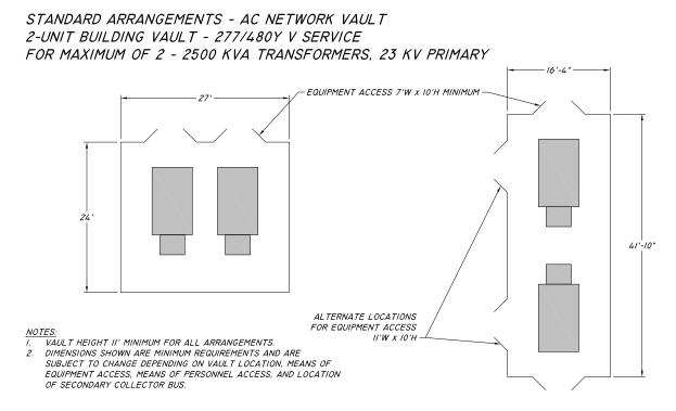
Figure 38 – Building & Free-Standing Vault Standard Arrangements, 2 – 2500 kVA, 23 kV
