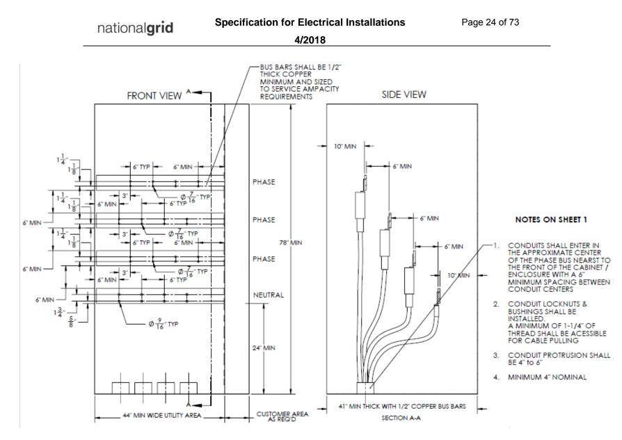
Figure 14 – 1000 to 1600 amperes Limiter Enclosure (Bottom Entry from Floor)
