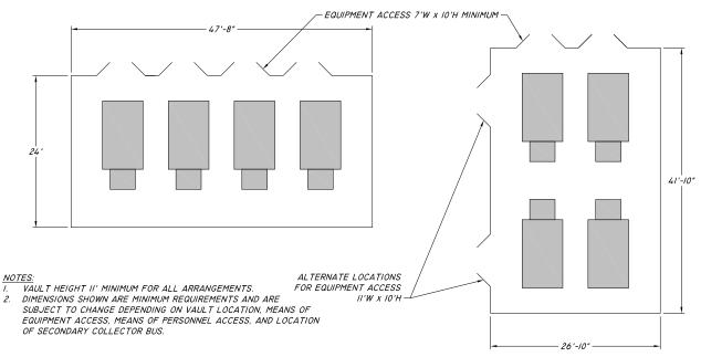
Figure 40 – Building & Free-Standing Vault Standard Arrangements, 4 – 2500 kVA, 23 kV
