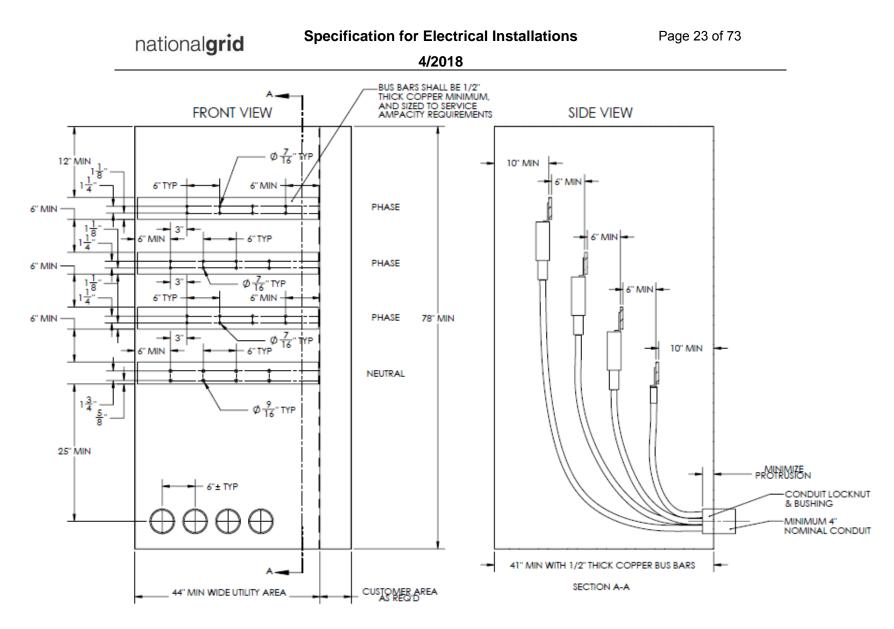
Figure 13 – 1000 to 1600 amperes Limiter Enclosure (Bottom Entry from Wall)
