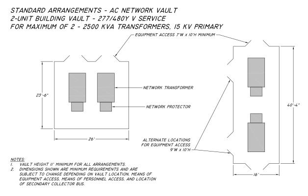
Figure 26 – Building & Free-Standing Vault Standard Arrangements, 2 – 2500 kVA, 15 kV
