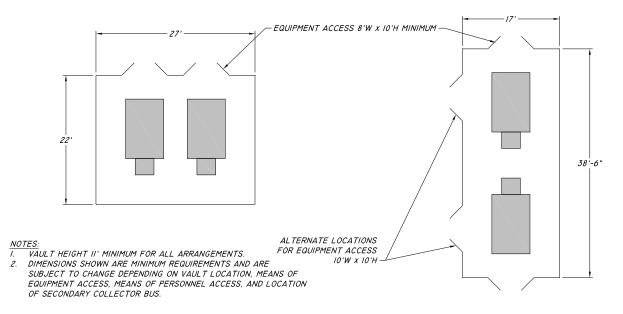
Figure 44 – Building & Free-Standing Vault Standard Arrangements, 2 – 2000 kVA, 34.5 kV
