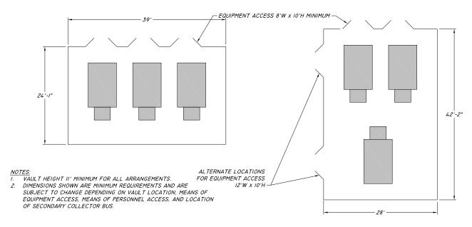
Figure 48 – Building & Free-Standing Vault Standard Arrangements, 3 – 2500 kVA, 34.5 kV
