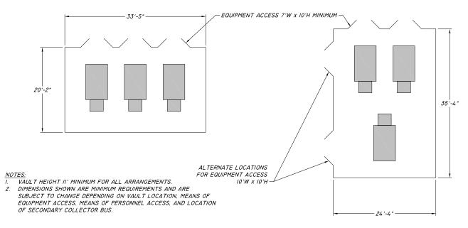
Figure 33 – Building & Free-Standing Vault Standard Arrangements, 3 – 1500 kVA, 23 kV
