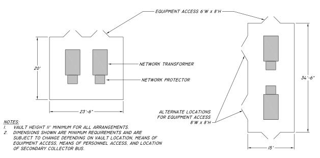
Figure 20 – Building & Free-Standing Vault Standard Arrangements, 2 – 1500 kVA, 15 kV
