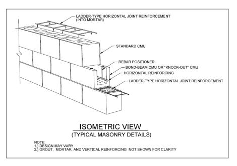
Figure 54 – CMU Wall Minimum Standards Isometric View
