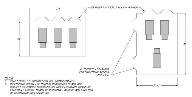
Figure 30 – Building & Free-Standing Vault Standard Arrangements, 3 – 1000 kVA, 23 kV
