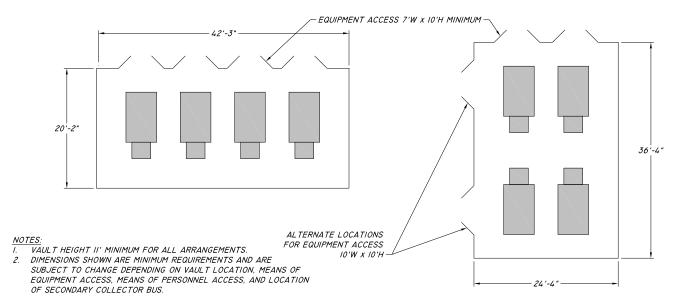
Figure 34 – Building & Free-Standing Vault Standard Arrangements, 4 – 1500 kVA, 23 kV
