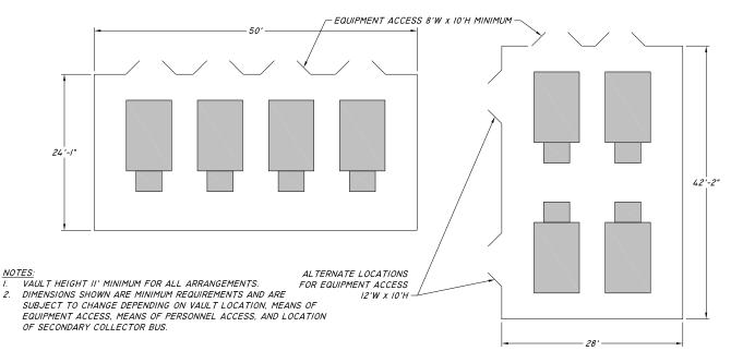
Figure 49 – Building & Free-Standing Vault Standard Arrangements, 4 – 2500 kVA, 34.5 kV
