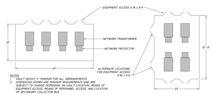
Figure 19 – Building & Free-Standing Vault Standard Arrangements, 4 – 1000 kVA, 15 kV
