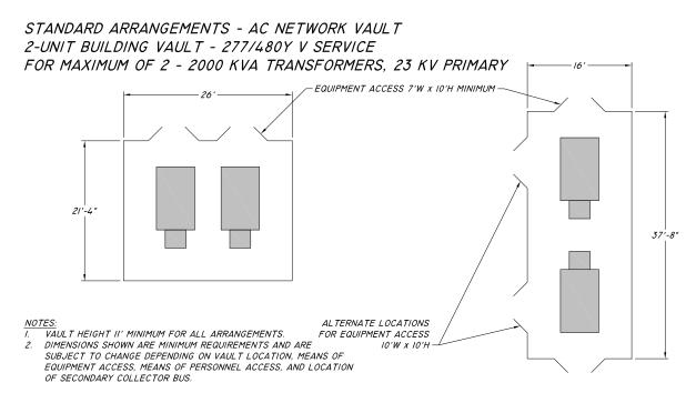
Figure 35 – Building & Free-Standing Vault Standard Arrangements, 2 – 2000 kVA, 23 kV
