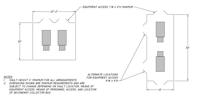
Figure 29 – Building & Free-Standing Vault Standard Arrangements, 2 – 1000 kVA, 23 kV
