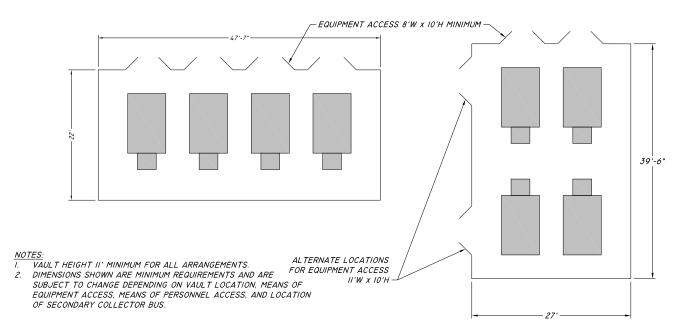
Figure 46 – Building & Free-Standing Vault Standard Arrangements, 4 – 2000 kVA, 34.5 kV
