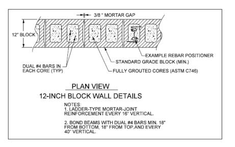
Figure 53 – CMU Wall Minimum Standards Plan View
